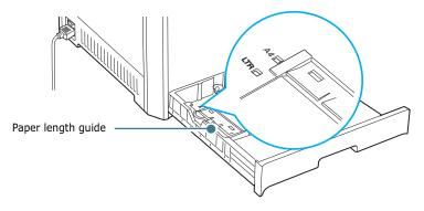
To remove the paper length guide, turn it slightly to your right to release the locks on the bottom of the guide, then pull it up.
